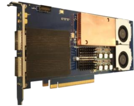
Accolade Technology ANIC Series FPGA based Network Adapters Advanced Deep Packet Capture & Analysis from 1 – 100G
